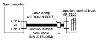
Ground the junction terminal block cable on the junction terminal block side with the standard accessory cable clamp fitting (AERSBAN-ESET). For the use of the cable clamp fitting, refer to Section 12.2.4, (2), (b).
